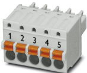
PCB connector, nominal current: 8 A, number of positions: 5, pitch: 3.81 mm, connection method: Push-in spring connection, color: light gray, contact surface: Tin
